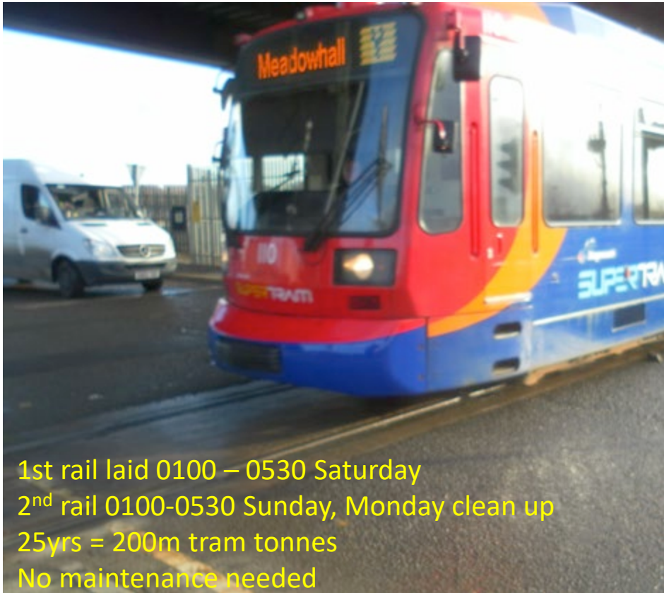
The LR55 installation, after girder rails failed in 6months
